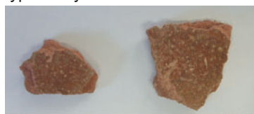
Magnesite flooring material showing typical red pink colouration
